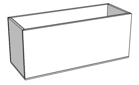
5) Finally, apply a thin layer of glue to the front edge of the enclosure. Set the front baffle in place on the glued edge. While ensuring all edges are even and square, position clamps to apply even pressure to all glued surfaces. Wipe away any glue squeeze-out on the outside of the enclosure. At this time double check that all edges are even and square (this cannot be adjusted once the glue is dry). Allow to dry according to the glue manufacturer's recommendations and remove clamps.
