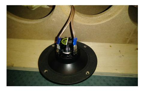
16) Connect woofer wires to 1st woofer terminals while observing polarity. Run a second set of wires from the 1st woofer's positive and negative terminals to the 2nd woofer's positive and negative terminals (parallel wiring, running two sets of woofer wires from the crossover is also an option). Set both woofers in place. Using a screwdriver, secure woofer with screws just until tight being careful not to strip out the holes (a power drill is not recommended).
