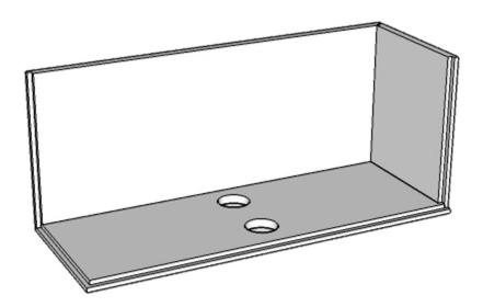
4) Next, glue all mating surfaces of the top panel and the other side panel and secure them in place with clamps so that even pressure is applied to all glued surfaces. Using a damp rag or paper towel wipe away any glue squeeze-out on the outside of the enclosure (excess glue on the inside is fine). Allow to dry according to the glue manufacturer's recommendations and remove clamps.
