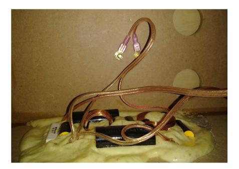
15) Connect tweeter wires to tweeter terminals while observing polarity (positive = wide terminal, negative = narrow terminal) and set tweeter in place. Using a screwdriver, secure woofer with screws just until tight being careful not to strip out the holes (a power drill is not recommended).
